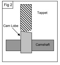
Even though cams with tapered lobes and tappets with a domed foot are not really "flat", they are lumped together with the cams and tappets that actually are flat under the general heading of "flat tappet cams and tappets".
