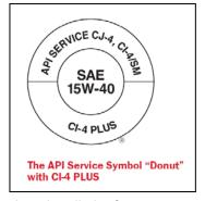
It is important to realize that none of these organizations specify exactly what goes into the oil; the focus is on how the oil performs. Oil from different companies may share the API "SM" service level designation, but each oil company uses their own blend of base oil and additives to meet those performance standards.
