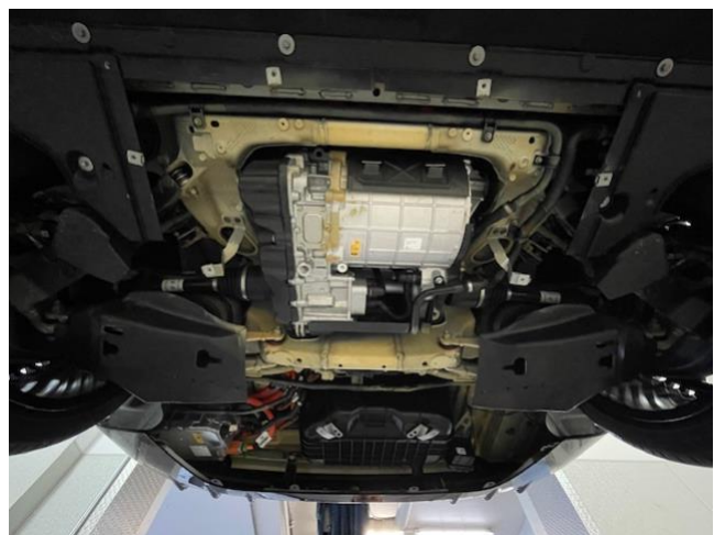
Looking aft, the electric drivetrain on the rear axle.
