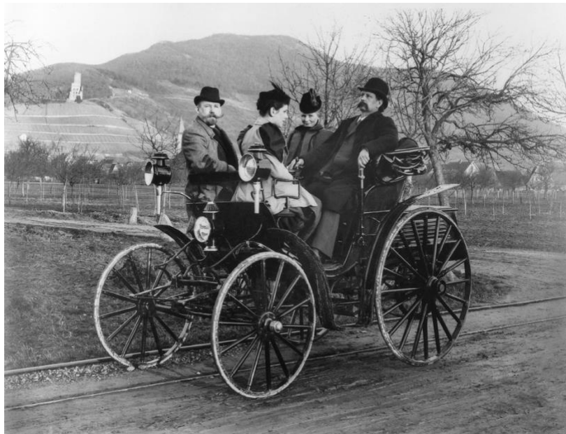
Carl and Bertha Benz in the back seat of a Benz Victoria, 1893. In the front her daughter Klara and Fritz Held. The Victoria was the first automobile with double-pivot steering, for which Benz applied for a patent on 28 February 1893. The invention is an essential prerequisite for the safe operation of a four-wheeled automobile: the risk of tipping over in curves is significantly reduced compared to turntable steering from carriage construction. (Photos on page 1 and 3 from Mercedes-Benz Classic Archives)
